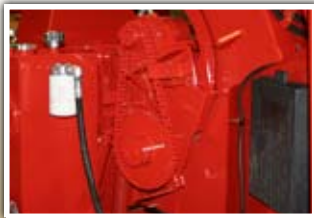
TORQMAX FEED WHEEL TorqMax Plus Top Feed Wheel Compression System with 2:1 torque amplification
